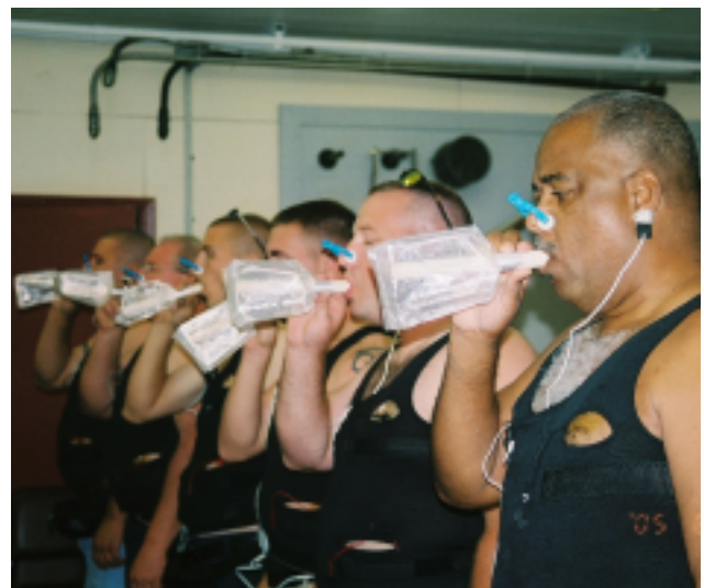
Calibration of the respiratory inductive plethysmograph function of the LifeShirt System
