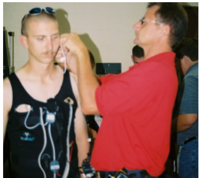
A MFRI instructor attaches the Nonin X-Pod pulse oximeter ear lobe sensor to a study participant.
